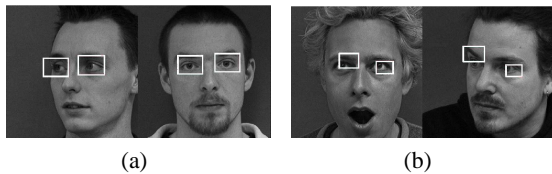
Figure 5: Eyes localized with less (a) and more (b) than a localization error of 0.2.
